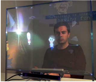
Figure 2. Gaze is used to reduce the transparency of the screen and illuminate the virtual environment.
